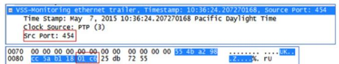
Figure 2: Example of Dual-byte port stamped in Wireshark.
